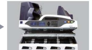
Removing jammed note and foreign object from the transport section
